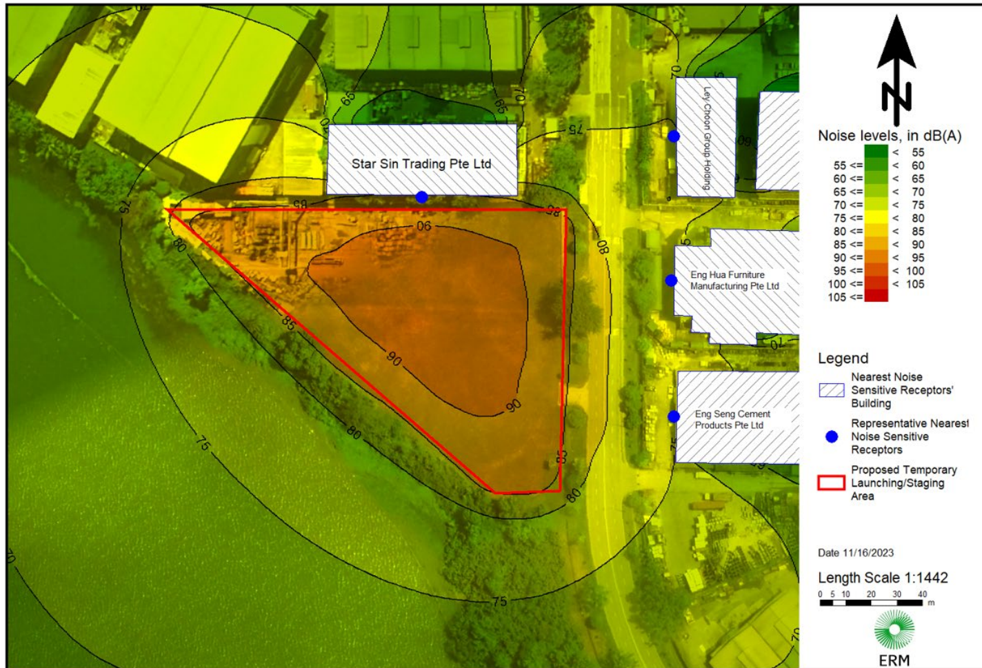
Figure 9-3: Unmitigated Noise Contours for the Proposed Temporary Staging Ground/ Launching Area and Integrated Project Substation (with O&M Facility)
