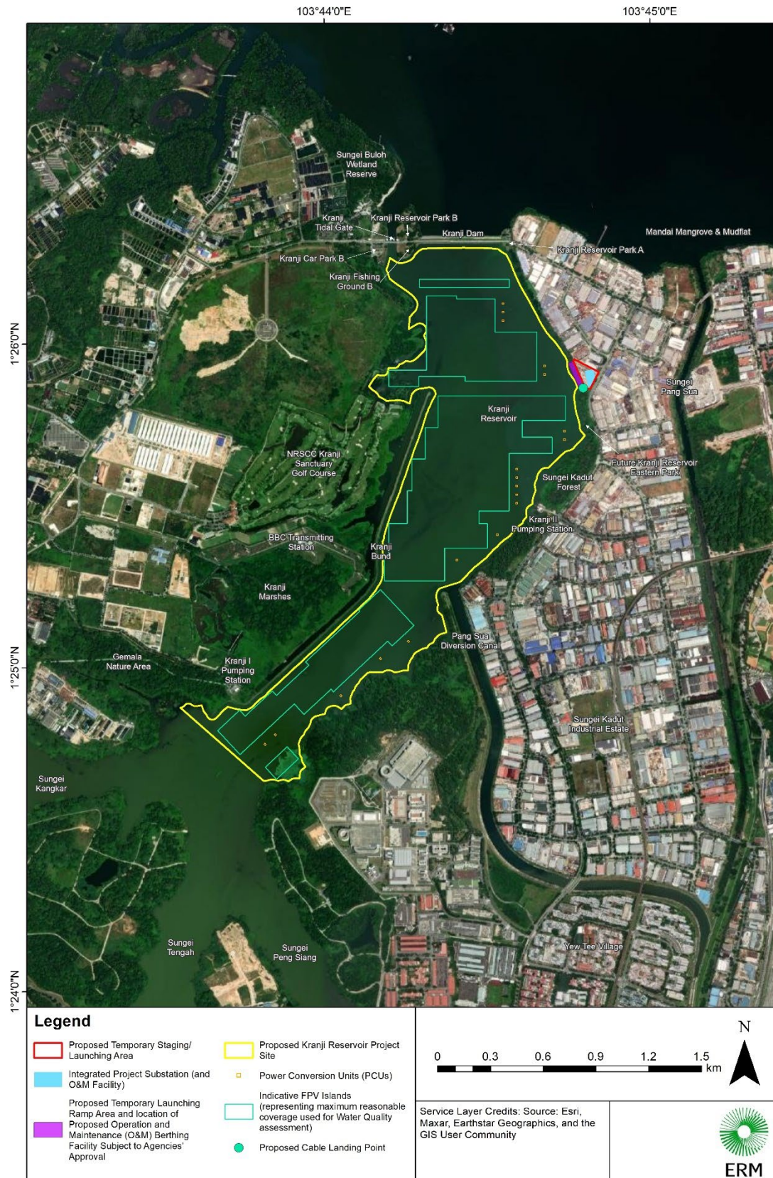
Figure 7-22: Unmitigated Maximum FPV Layout (25 western shoreline setback to FPV panels) Considered in the Pre-mitigation Biodiversity Impact Assessment
