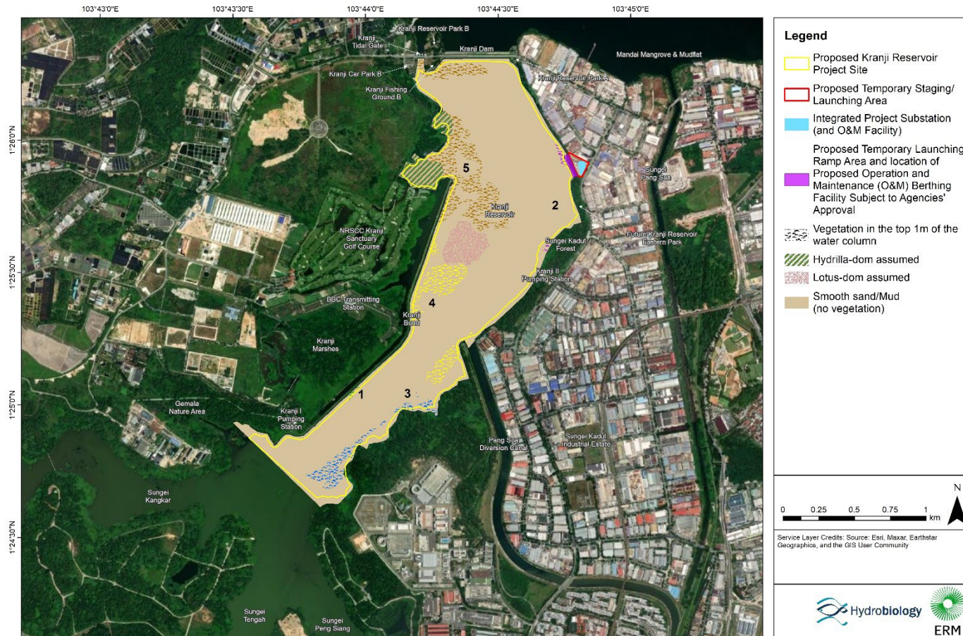
Figure D-3 Map of vegetation within top 1m of the water column in the Reservoir Project Site area. Numbers and different colours indicate nominal zones for biomass calculations
